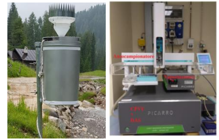
On the left: Rain gauge installed in Valfredda; on the right: the Picarro instrument used for the water isotopes analyses at Ca'Foscari.
