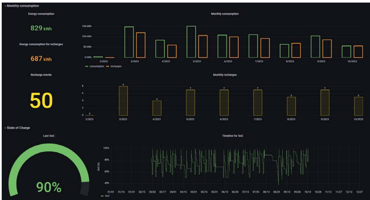
Figure 8 Grafana Dashboard for Electric Vehicle Fleet Monitoring (Vehicle 6)
