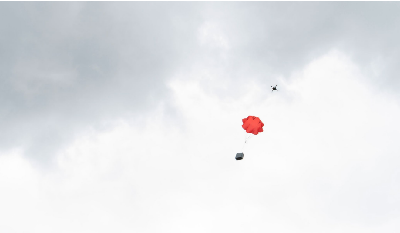
A drone delivering first aid to within 10 m of the accident site, a small parachute slows the drop of the load.
