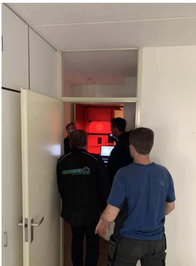
Figure 85 Blower-door test in an unoccupied apartment in Marienheувel, Soest
