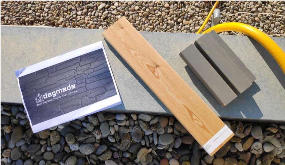
Figure 111 The different types of finishing considered for the timber external cladding (from left to right); Yakisugi treatment (burn timber surface as external protection), thermo-treated (heat treatment to improve timber stability), grey colored coating for protection.
