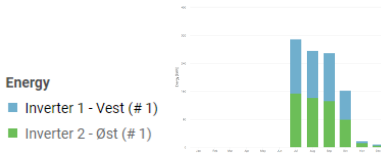
Figure 47: PV production during 2018. The PV panels were fully operational from July
