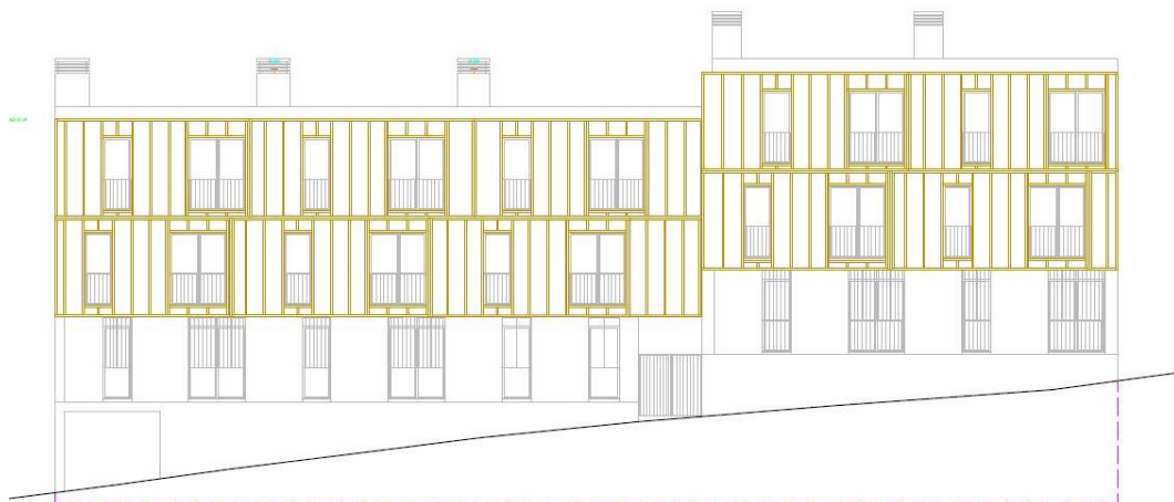
Figure 95. Structural composition of the PMF with the final 10 panels horizontal panels division
