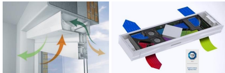
Figure 89. Mechanical Ventilation unit of the PMF facade
