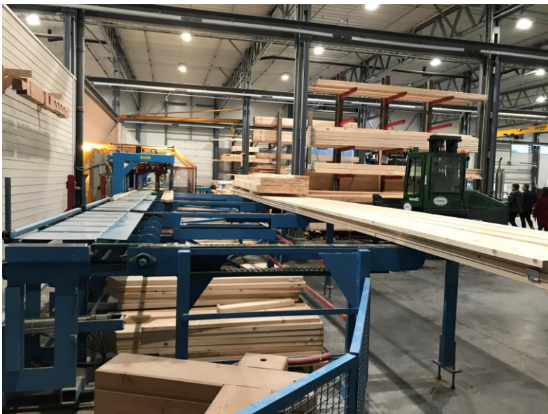
Figure 20: Lindal's CNC saw for precutting of studs and beams
