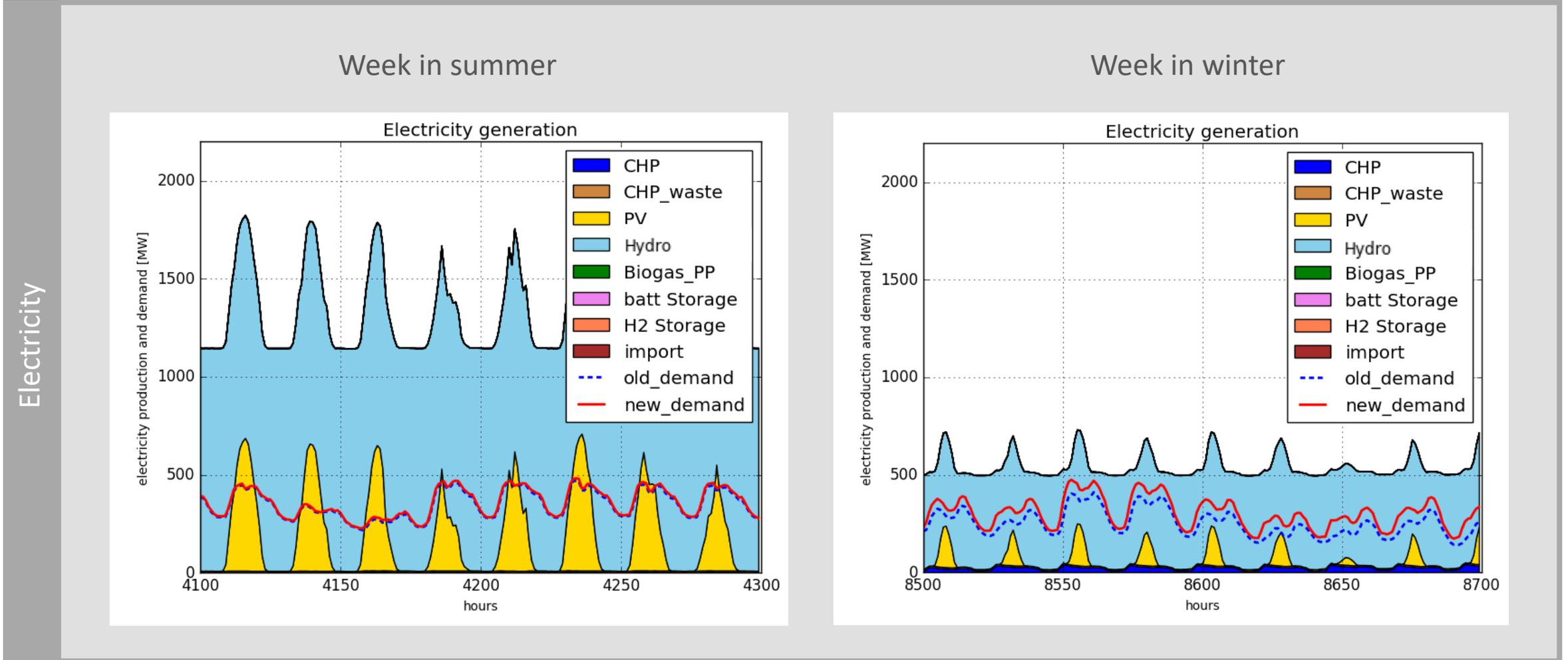
The electricity consumption increases and the profiles changes due to the use of heat pumps
