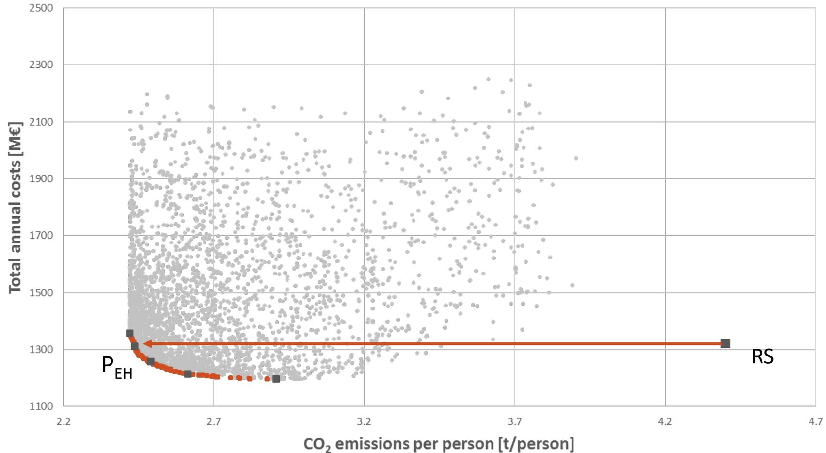
Each point of the cloud represents a specific combination of technologies in the year 2050 with related costs and CO<sub>2</sub> emissions. The P<sub>EH</sub> scenario represents a combination of technologies with annual costs similar to the reference scenario (current combination of technologies), but with heavily reduced emissions.
