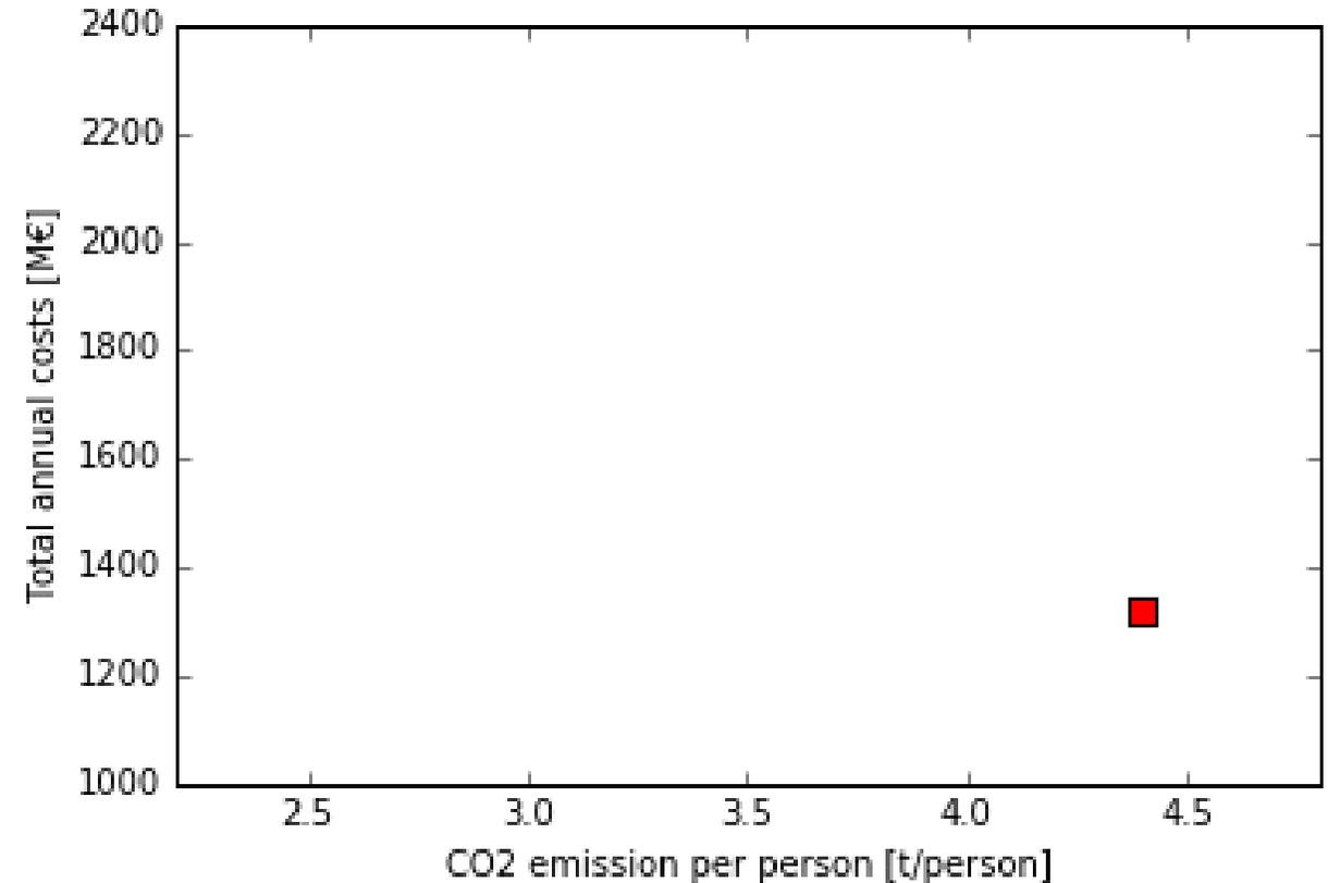
Each point on the chart shows total costs and CO<sub>2</sub> emissions per each energy system. For each energy system, hourly energy production and consumption have been simulated.
