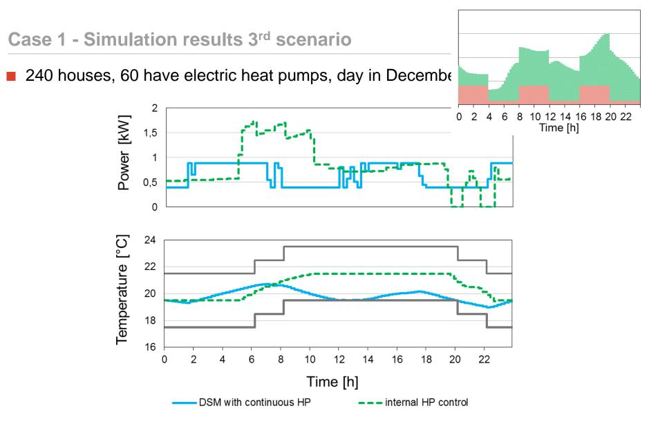
Continuous HP: 5 houses with HP always ON; 13 houses with HP ON for 23 hours
