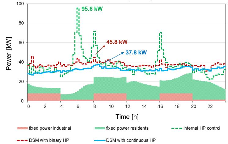
with the continuous HP operation, almost 75% of heat pump consumption is reallocated during the peak time
