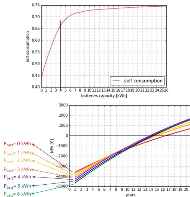
Figure 28 Sizing of the best battery capacity coupled to a rooftop residential 3 kWp PV system.
