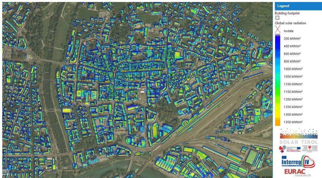
Figure 13 PV potential estimated through the Solar Tyrol project webGIS [49].
