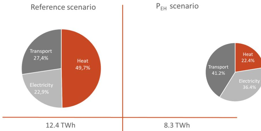
Figure 19 Comparison of the overall energy consumption between the reference scenario and the P<sub>EH</sub> scenario.
