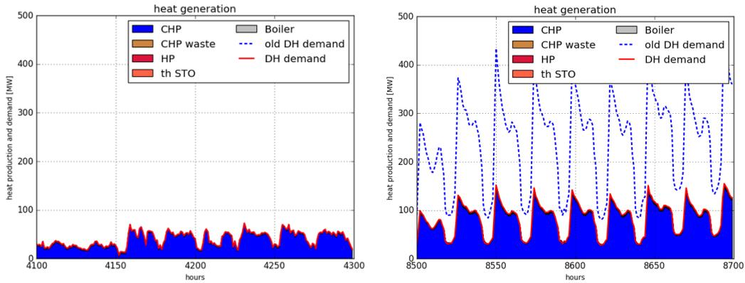
Figure 24  $P_{EHT}$  scenario. Hourly heat production in the district heating network of a week in June (from 4100 to 4300) and of a week in December (from 8500 to 8700).
