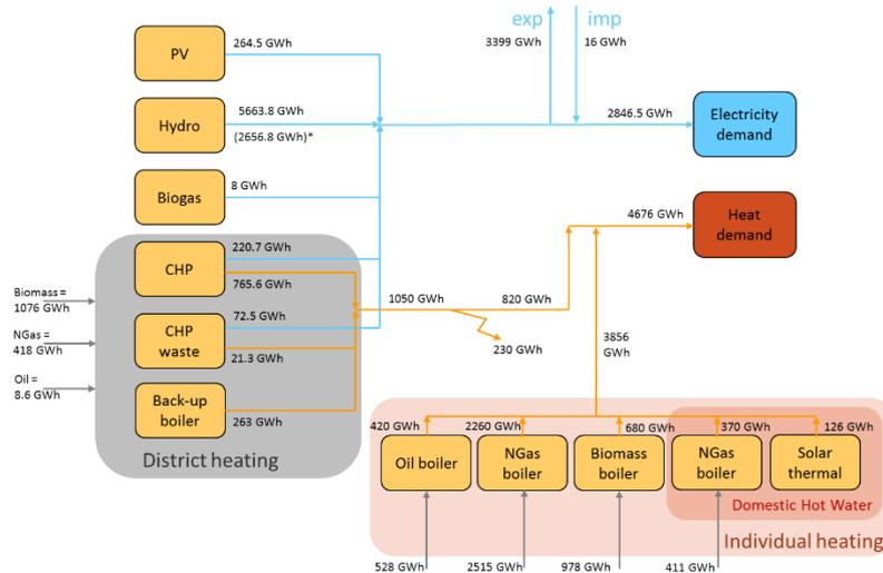
Figure 5 Diagram of the electricity and thermal sector of the South Tyrol energy system.
