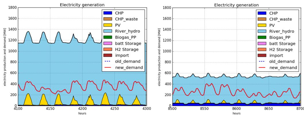
Figure 11 Reference scenario 2014 South Tyrol. Hourly electricity production of a week in June (from 4100 to 4300) and of a week in December (from 8500 to 8700).
