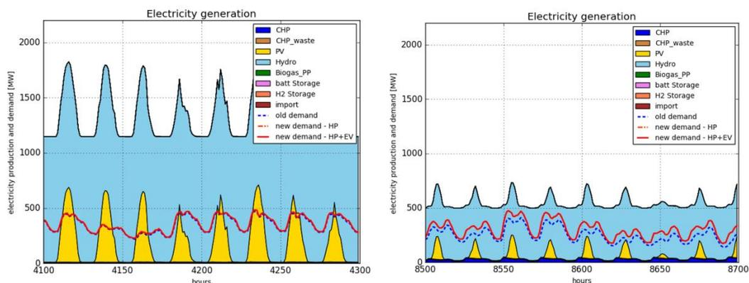
Figure 16 P<sub>EH</sub> scenario. Hourly electricity production of a week in June (from 4100 to 4300) and of a week in December (from 8500 to 8700).
