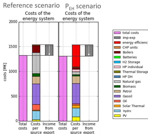
Figure 20 Comparison between the total annual costs of the reference scenario and the P<sub>EH</sub> scenario.
