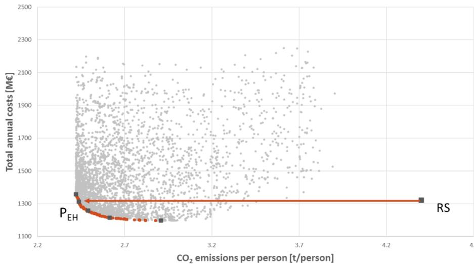
Figure 15 Pareto front of best configuration of the energy system of the South Tyrol province.
