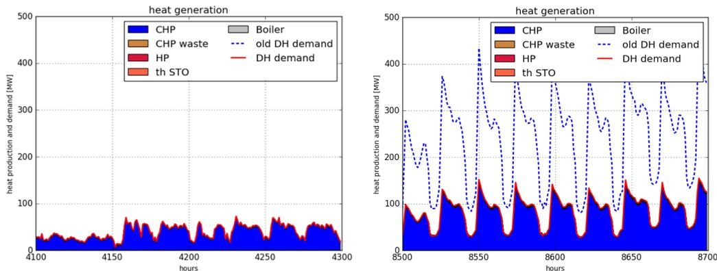
Figure 18 P<sub>EH</sub> scenario. Hourly heat production in the district heating network of a week in June (from 4100 to 4300) and of a week in December (from 8500 to 8700).
