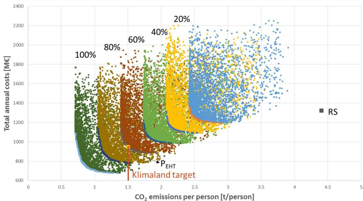
Figure 21 Pareto fronts with different levels of penetration percentage of zero emission transport on the overall kilometers covered in the transportation sector.
