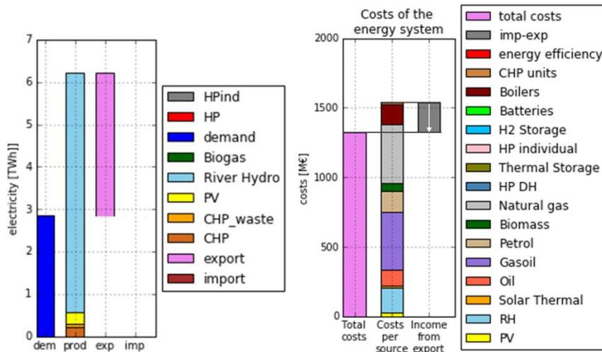
Figure 10 Annual electricity balance, on the left, and total annual costs balance for the energy system baseline.
