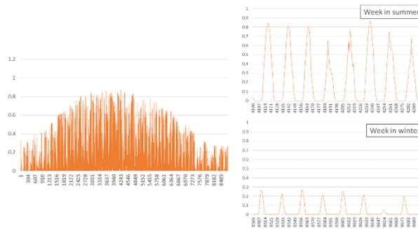
Figure 8 Hourly distribution of photovoltaics electricity production.
