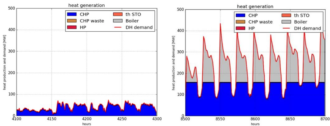
Figure 12 Reference scenario 2014 South Tyrol. Hourly heat production in the district heating network of a week in June (from 4100 to 4300) and of a week in December (from 8500 to 8700).
