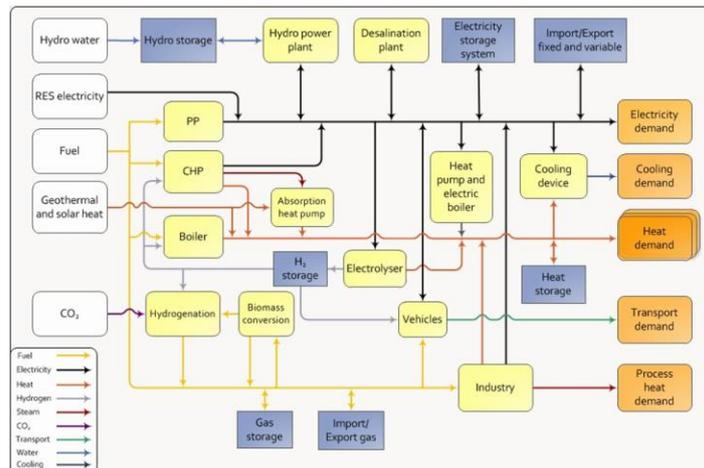
Figure 1 - Diagram of the EnergyPLAN's structure.
