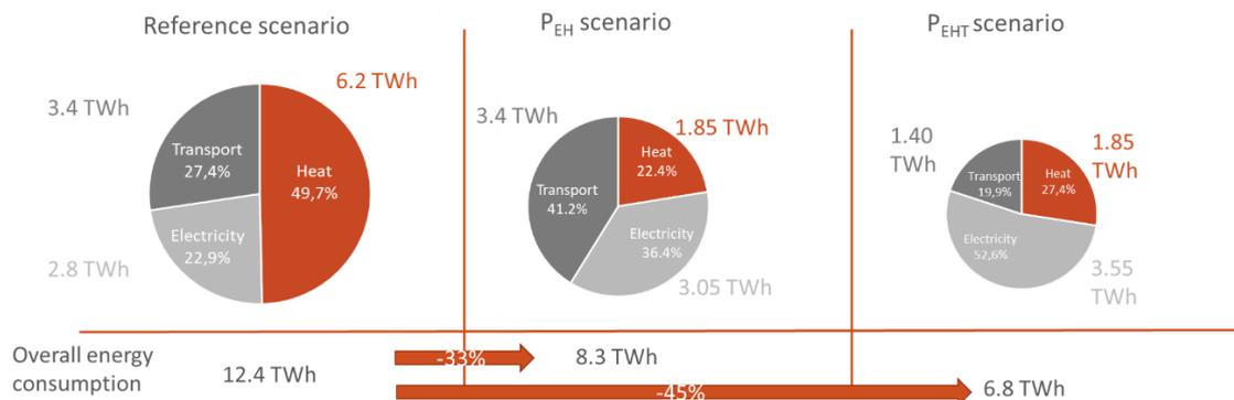
Figure 25 Comparison of the overall energy consumption between the reference scenario, the  $P_{EH}$  and the  $P_{EHT}$  scenario.
