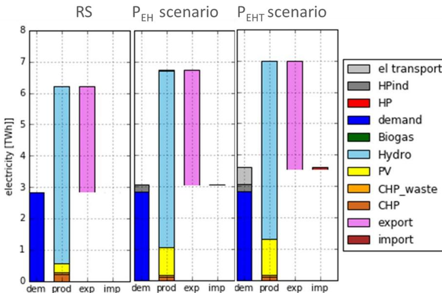
Figure 23 Annual electricity balance, comparison between the reference scenario and the  $P_{EHT}$  scenario.
