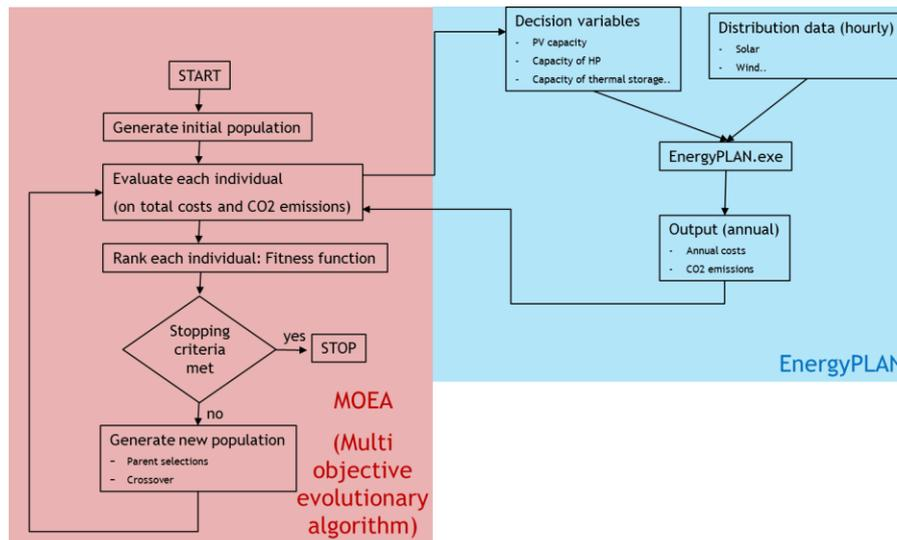
Figure 3 Diagram of the EPLANopt model.
