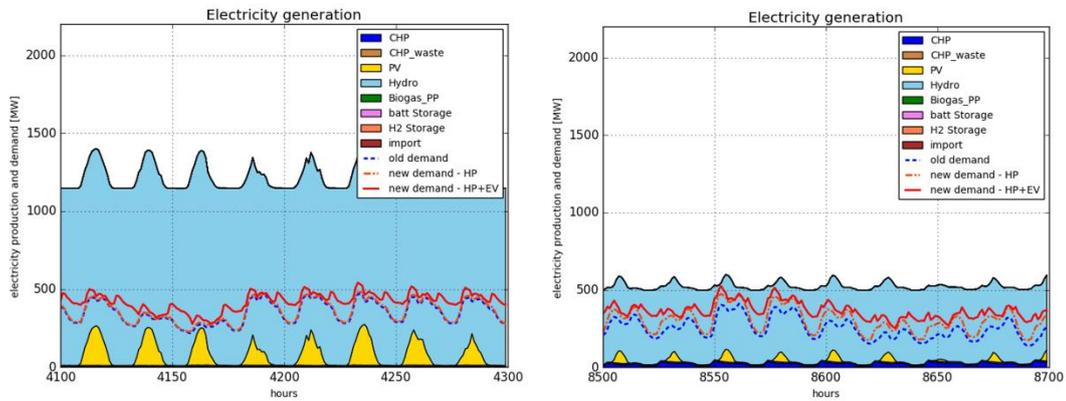
Figure 22  $P_{EHT}$  scenario. Hourly electricity production of a week in June (from 4100 to 4300) and of a week in December (from 8500 to 8700).
