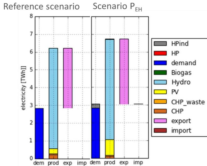
Figure 17 Annual electricity balance, comparison between the reference scenario and the P<sub>EH</sub> scenario.
