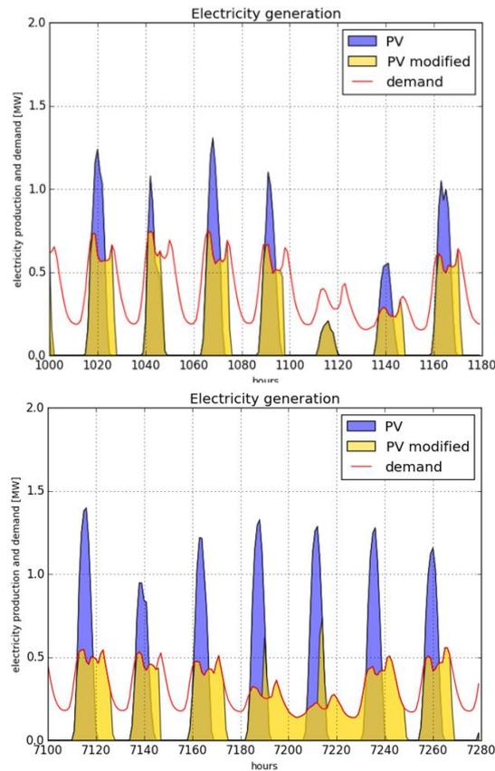
Figure 29 Sizing of the best battery capacity coupled to a rooftop residential 3 kWp PV system and the final production profile.
