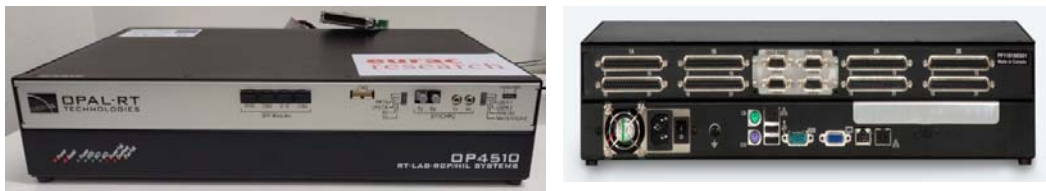
Figure 3 – Real Time Simulator (RTS) OPAL- RT 4510 hardware
