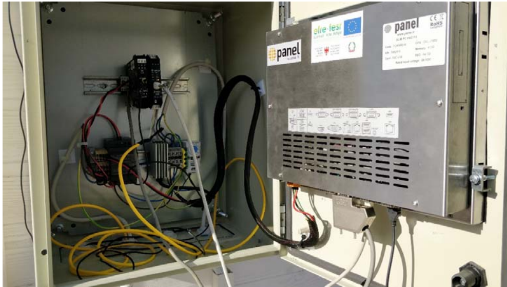
Figure 21 - Z-LINK receiver and Z-KEY transformer, and the respective connections to the PC
